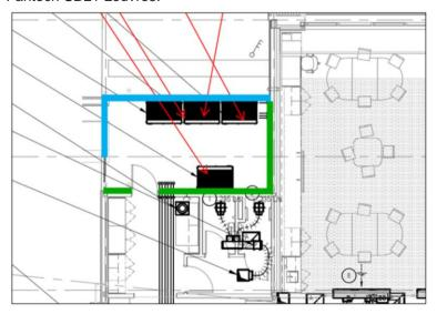
Install acoustic absorption to the walls of the plant area for the extent shown in GREEN below. This
